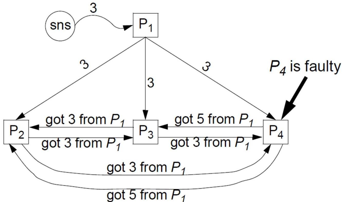
The two non-faulty processors  $P_2$  and  $P_3$  agree on value 3, which is the value produced by the non-faulty input unit  $P_1$ .
