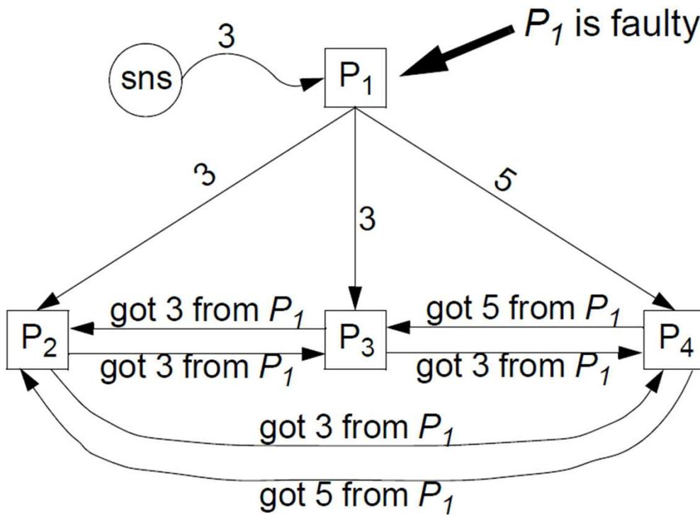
P<sub>2</sub>, P<sub>3</sub>, and P<sub>4</sub> will reach agreement on value 3, despite the faulty input unit P<sub>1</sub>.
