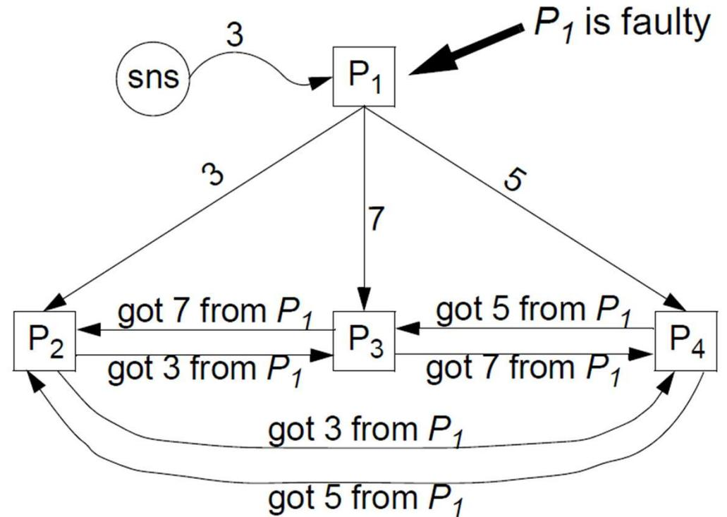
P<sub>2</sub>, P<sub>3</sub>, and P<sub>4</sub> will reach agreement on the default value, e.g. 0 (used when no majority exists), despite the faulty input unit P<sub>1</sub>.
