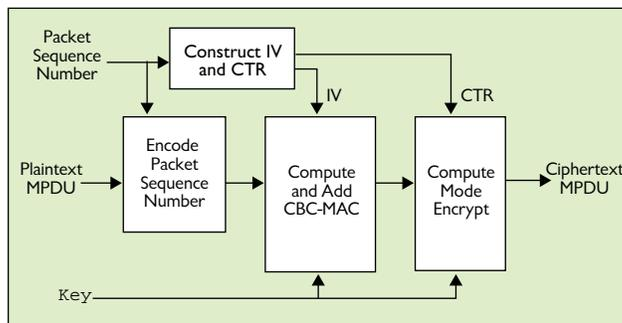
**Figure 2. CCM Mode provides confidentiality and integrity.**
