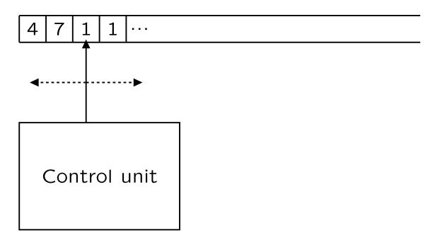
The TM uses the (infinite) tape as a read-write memory with unrestricted access.
