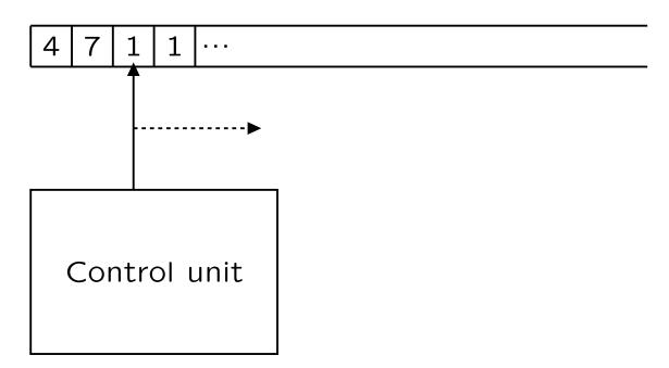
We can read the input sequentially. The control unit has a finite number of states, which is the only memory.
