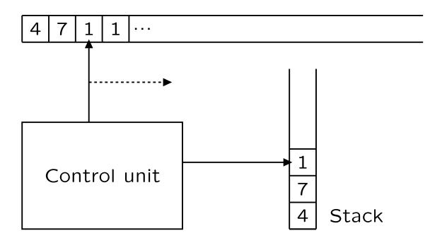
The PDA is an FA that has unlimited memory with restricted access in the form of a stack.
