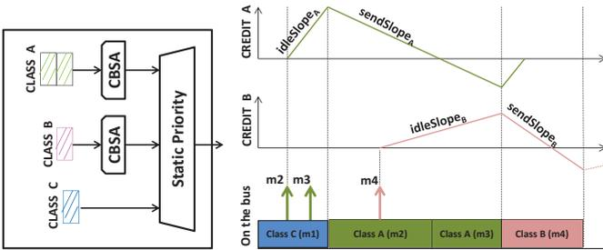
Fig. 1. Snapshot of an exemplary AVB switch.
