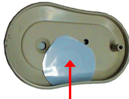
Semantic Product Memory Chip in the backcover plastic frame with product specification
