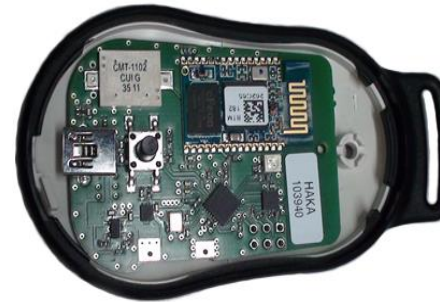
Bluetooth circuit board with keyfinder logic packaged inside a plastic shell
