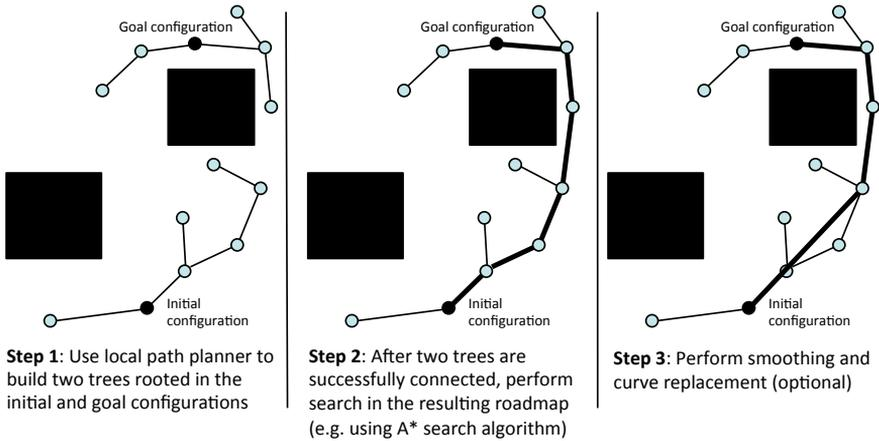
Figure 4.6: Example execution of RRT in a simple 2D environment.
