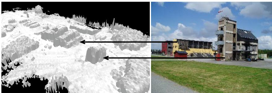
Figure 6.9: Overview of the reconstructed elevation map of the Revinge flight test area based on the laser range finder data (left) and a photo of corresponding building structures (right).
