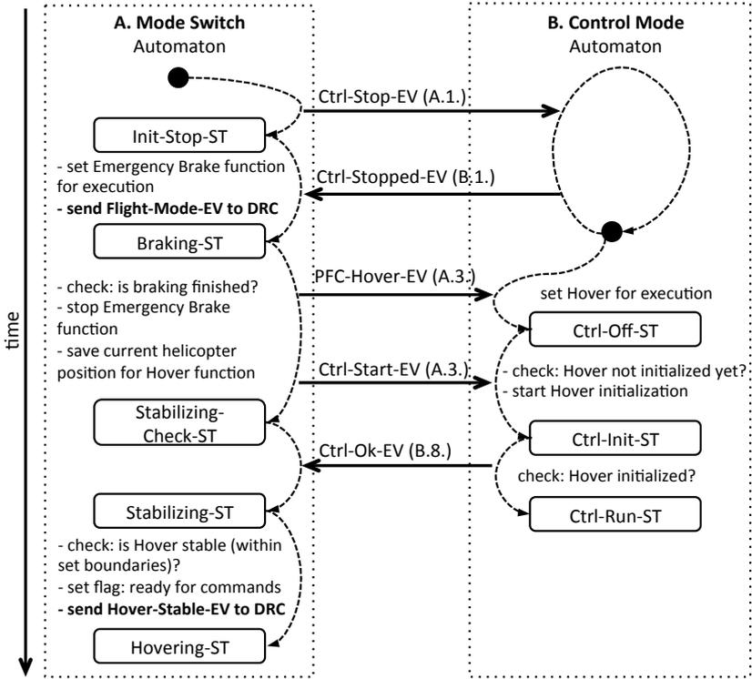
Figure 3.9: An execution trace for use case 1 showing the interaction between the *Control Mode* and the *Mode Switch* automata.
