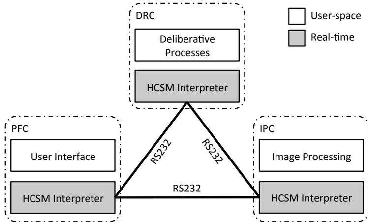
Figure 3.5: Overview of the HCSMs used in the UASTechLab RMAX UAV platform.
