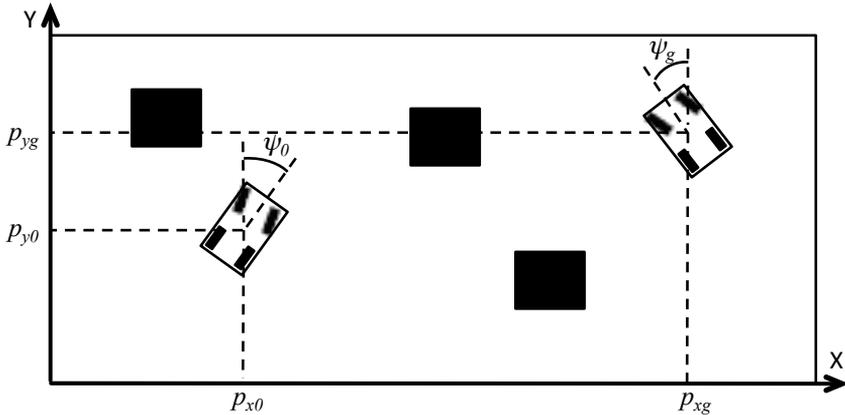
Figure 4.1: An example of a car-like robot path planning problem.
