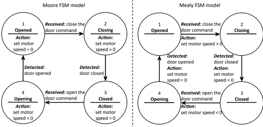
Figure 3.1: An example of a simple four-state system for an elevator door using Moore and Mealy FSMs.
