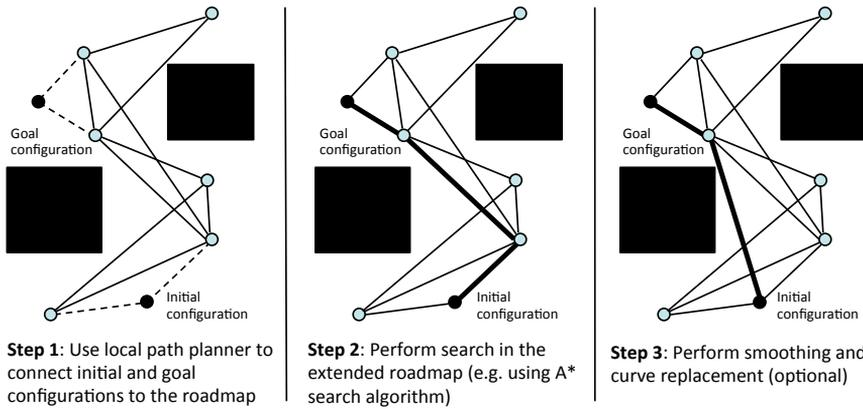
Figure 4.3: An example of the PRM online phase for a simple 2D environment.
