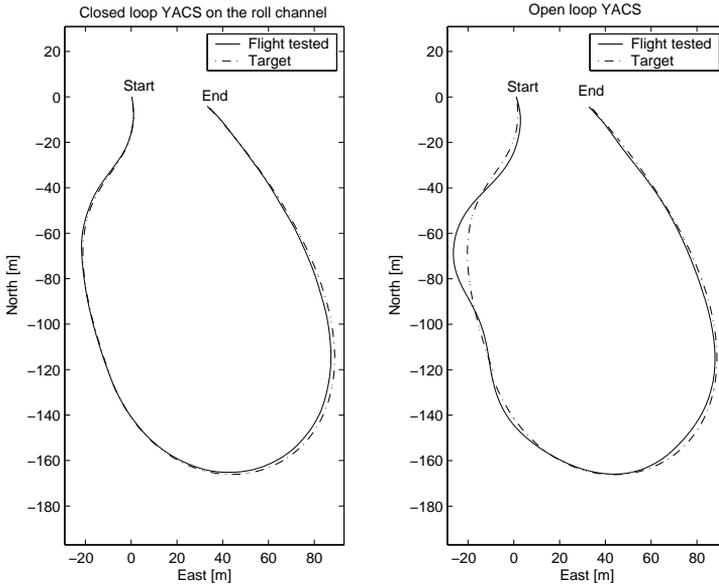
Figure 2.12: Comparison of path tracking performance using two different roll controllers performed at 36 km/h constant velocity.
