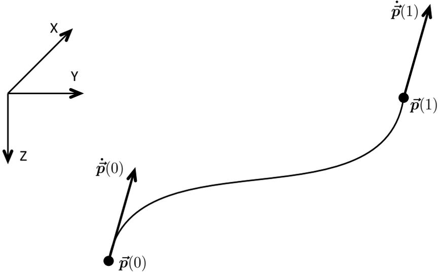
Figure 2.9: Boundary conditions for a path segment.
