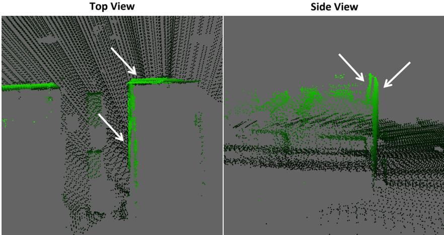
Figure 6.8: Examples of measurement errors in a single point cloud.
