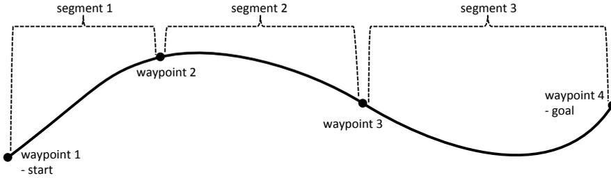
Figure 2.6: Example path consisting of three segments.
