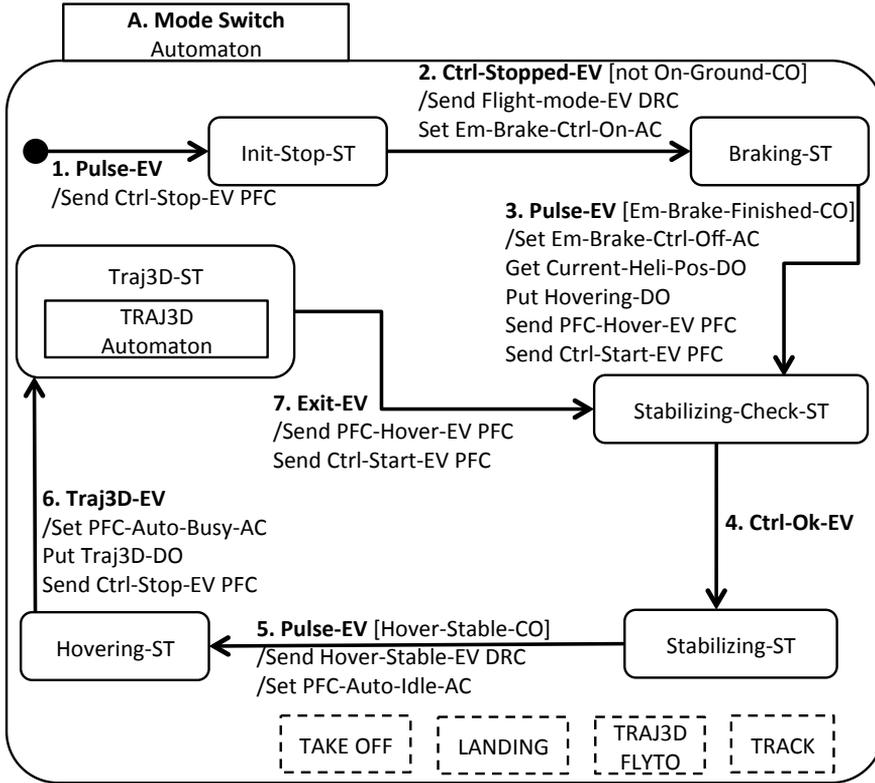
Figure 3.8: The *Mode Switch* automaton. Simplified view focused on a path following control mode execution.
