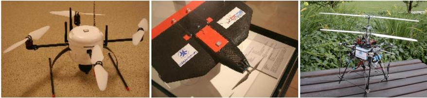
Figure 2.1: From left to right: LinkQuad (a quadrotor platform); PingWing (a fixed wing platform); LinkMAV (a coaxial helicopter).
