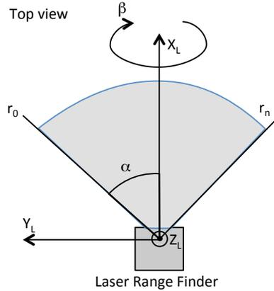
Figure 6.4: Polar and Cartesian coordinate systems of the laser range finder.
