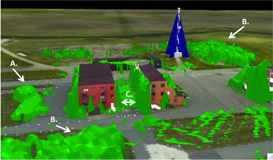
Figure 6.11: Overlay of the new elevation map with the existing Revinge flight test area model.
