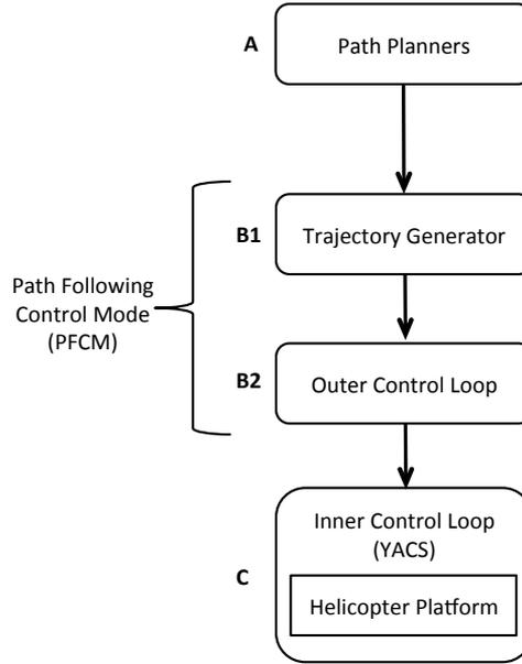
Figure 2.7: The path following control mode and its components.
