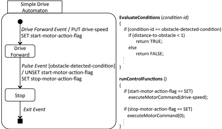
Figure 3.4: An example of a simple HCSM modelling a driving behaviour of a ground robot platform.
