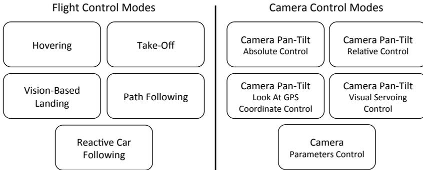
Figure 1.2: Control modes implemented on the UASTechLab RMAX helicopter platform.
