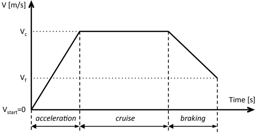
Figure 2.11: Example of an ideal velocity profile for a straight line path.
