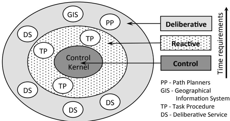
Figure 2.4: The UASTechLab hybrid deliberative reactive architecture.
