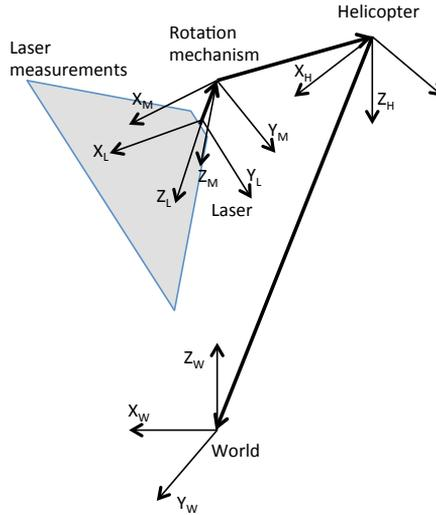
Figure 6.3: Coordinate systems used in the scan transformation in the UASTechLab RMAX platform.
