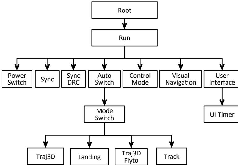
Figure 3.6: The hierarchical view of the HCSM automata running on the PFC computer.
