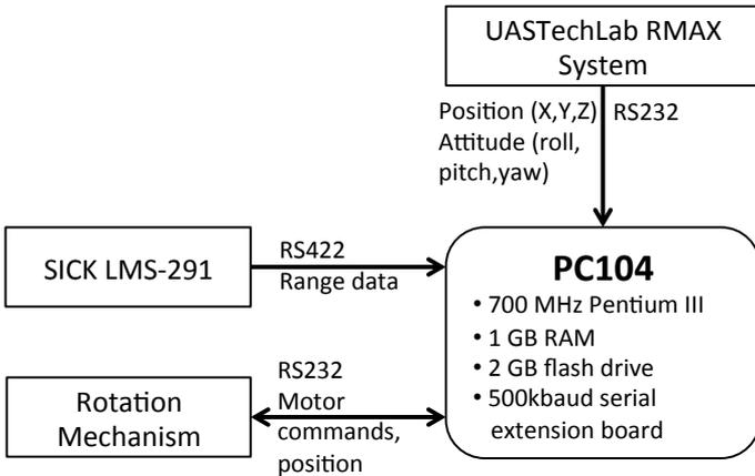
Figure 6.2: A photograph and schematic of the integration of the rotating laser range finder sensor with the UASTechLab RMAX UAV.
