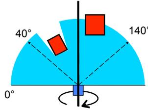
Figure 6.1: Top view of the SICK LMS-291 scanning field and the axis of rotation when using the rotation mechanism.
