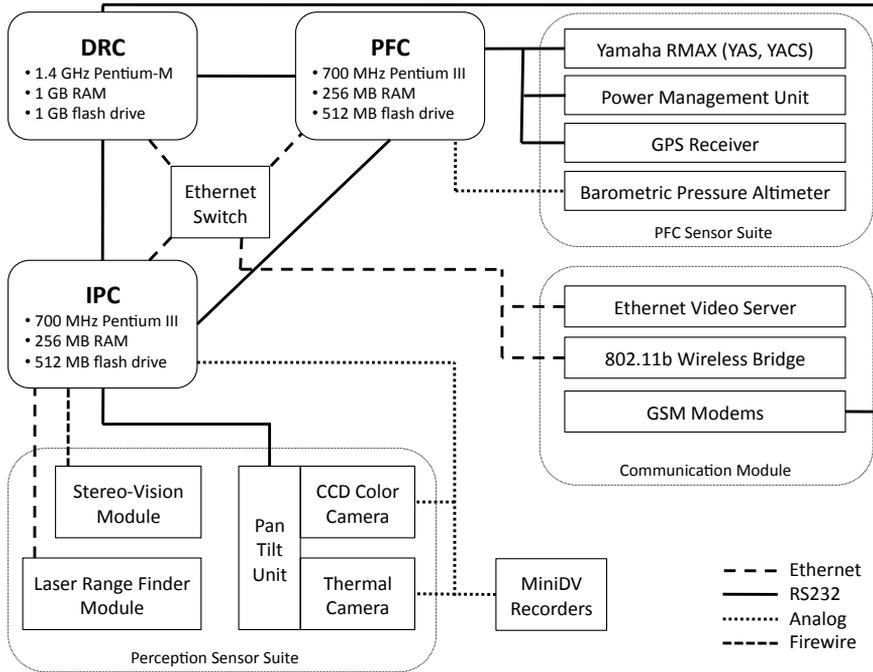
Figure 2.3: On-Board Hardware Schematic.
