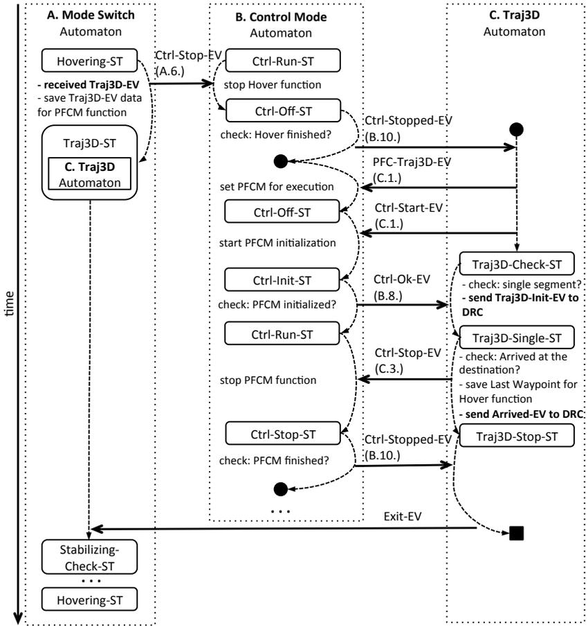
Figure 3.12: An execution trace for use case 2 showing the interaction between the *Control Mode*, the *Mode Switch* and *Traj3D* automata.
