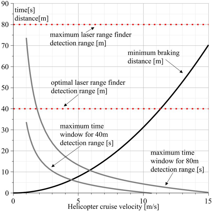
Figure 6.13: The minimal braking distance and time windows for the UASTechLab RMAX UAV as a function of the cruise velocity.
