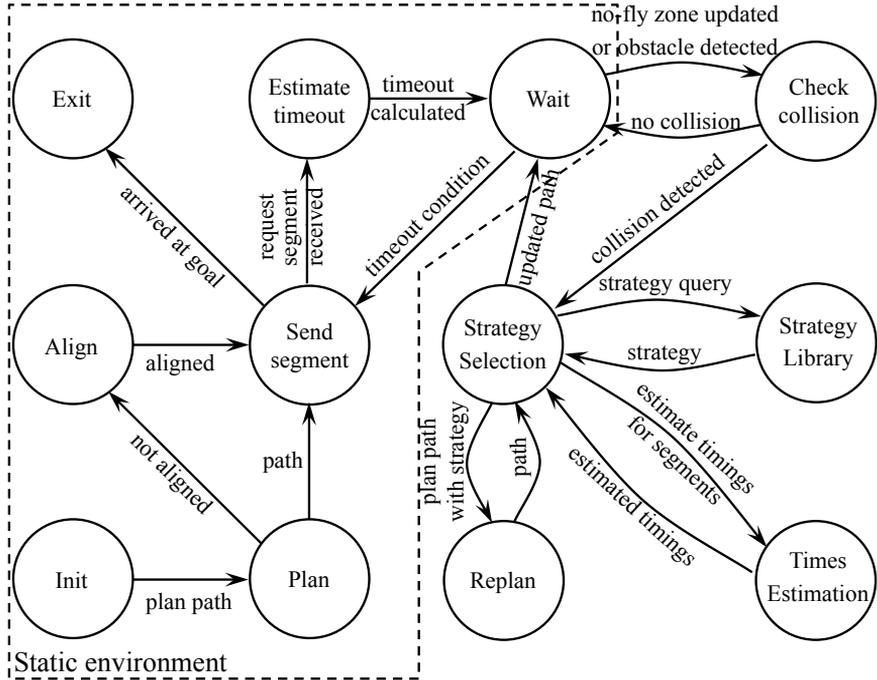
Figure 4.8: The dynamic path replanning automaton.
