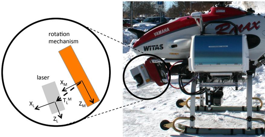
Figure 6.5: Displacement between the laser range finder and the rotation mechanism.
