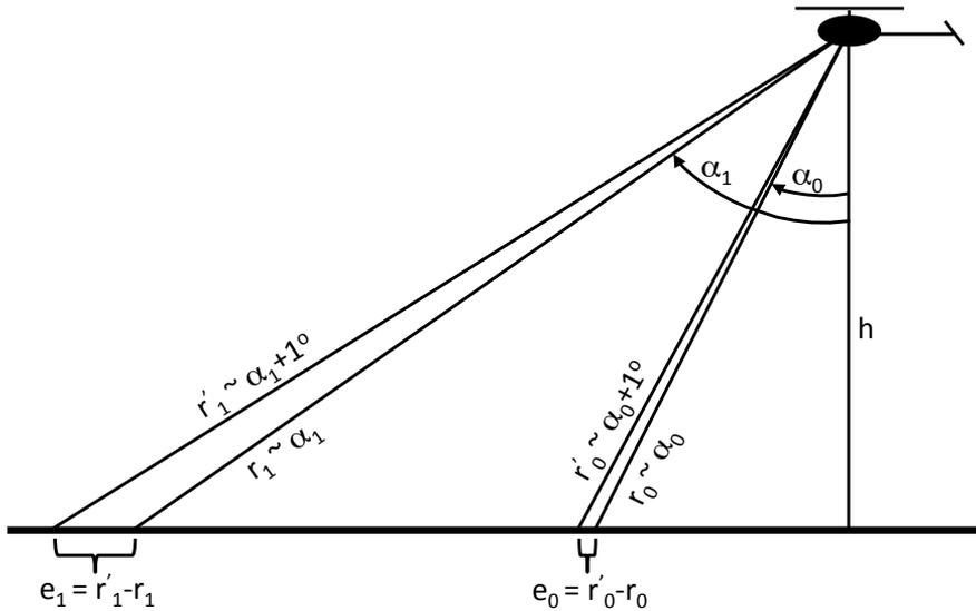
Figure 6.6: A simplified example of the influence of pitch angle uncertainty on the LRF measurement error.
