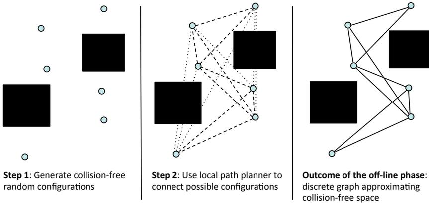
Figure 4.2: Example PRM roadmap generation (offline phase) for a simple 2D environment.
