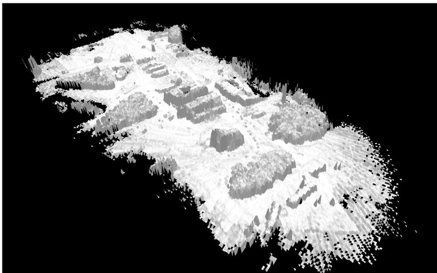
Figure 6.10: Reconstructed elevation map of the Revinge flight test area based on the laser range finder data.
