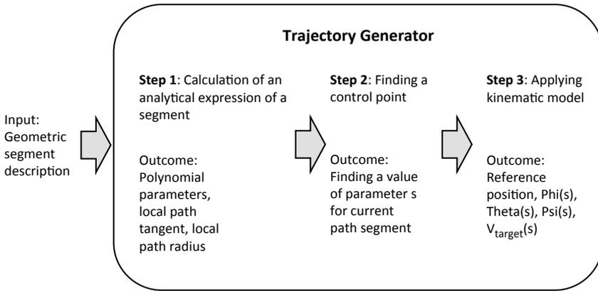
Figure 2.8: Calculations performed by the trajectory generator.
