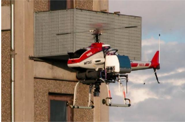
Figure 1.1: The UASTechLab RMAX helicopter platform.
