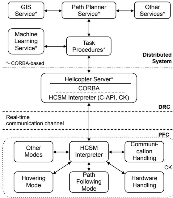
Figure 2.5: Navigation subsystem and main software components
