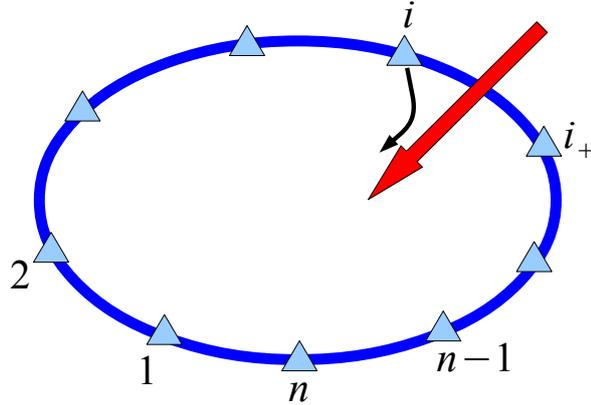
Figure 1: Perimeter guarding UAVs; an intrusion of the perimeter segment between UAVs  $i$  and its adjacent UAV  $i_+$
