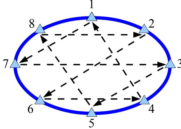
Figure 4: Optimal replacement sequence for 8 UAVs
