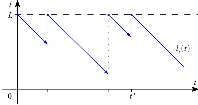
Figure 2: Charge of UAV  $i$  vs. time
