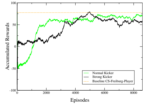
Fig. 17. Learning to improve pre-learned skills and their selection while competing with a hand-crafted player. If equipped with a different kicking device (normal kicker), the robot adapts its strateg.
