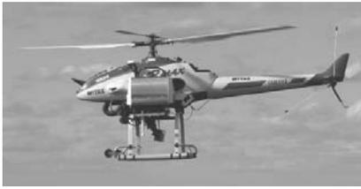
Figure 2: The WITAS UAV platform.
