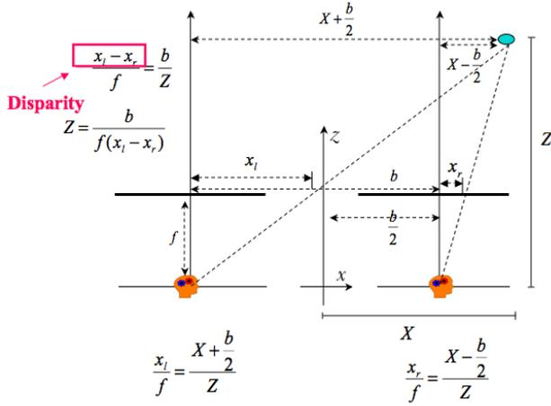
Fig. 1. Stereo disparity principle for parallel cameras.
