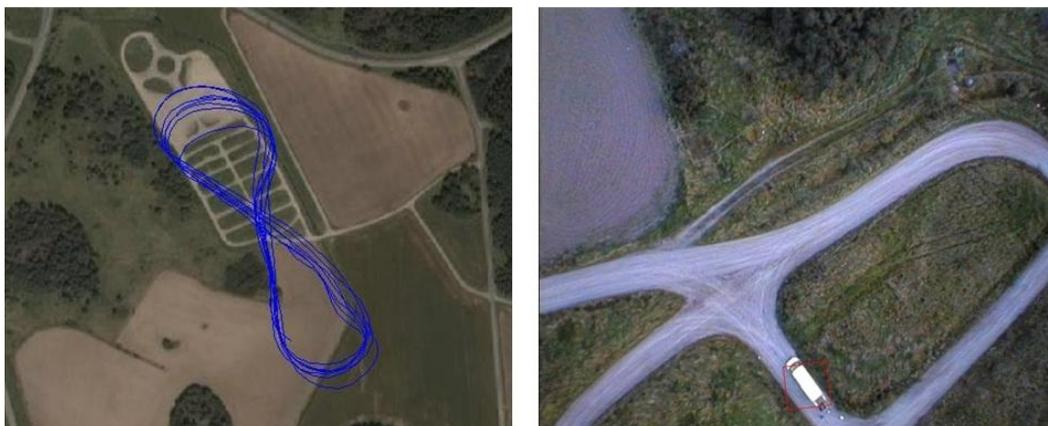
**Figure 7.** On the left picture is displayed the MAV's flight path during the ground object localization task. On the right, the ground object is automatically tracked in the image (red square).
