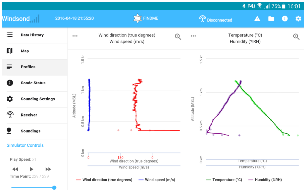
Figure 1. The line graphs already present in the app when work started. Note the zoom button to the top right of each graph, which allows you to let that one graph cover the entire screen.
