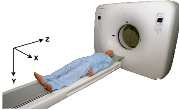
Figure 3.2: A CT scanner with a patient and the DICOM Patient Space Coordinate System. <sup>5</sup>
