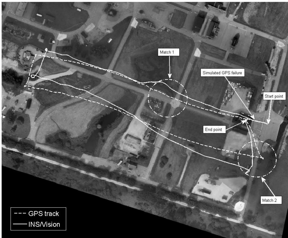
Figure 9. Vision-aided navigation experiment using image registration for position drift compensation.
