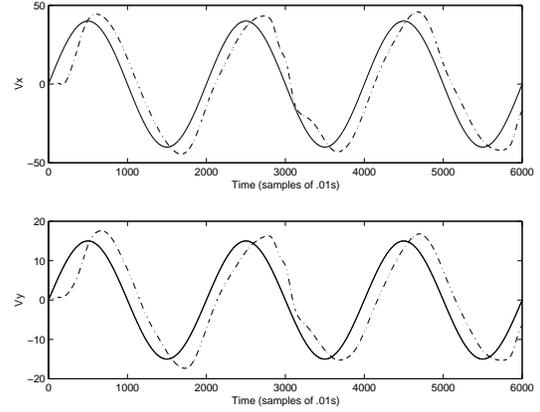
Figure 3: Velocity tracking with strong wind action, desired – and actual -.- .
