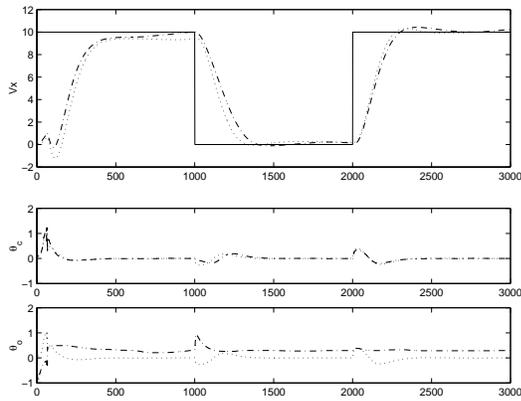
Figure 5:  $\dot{x}$  set-point change, desired – , strong -.- and weak ... wind and control inputs.
