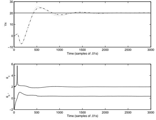
Figure 2: Upper-part: High  $\dot{x}$ -velocity set-point regulation with strong and weak wind action, desired – , strong -.- and weak ... wind. Lower-part: Control inputs for strong – and weak ... wind.
