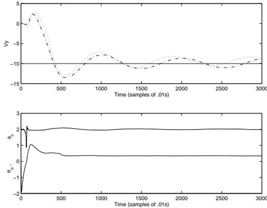
Figure 1: Upper-part: Low  $\dot{y}$ -velocity set-point regulation with strong and weak wind action, where desired – , strong wind -.- and weak ... wind. Lower-part: Control inputs for strong – and weak ... wind.
