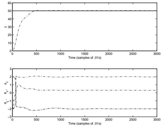
Figure 7: Altitude set-point regulation, desired – and actual -.- and control inputs.
