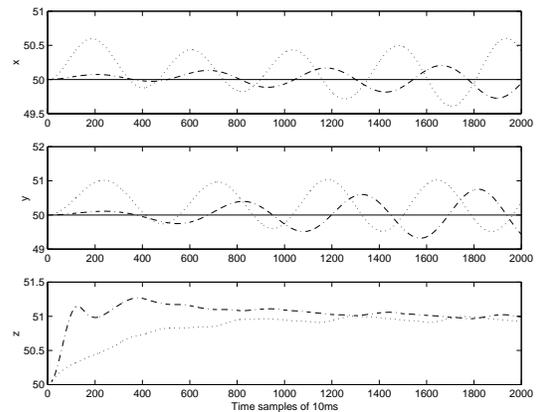
Figure 9: Hovering with strong and weak wind, desired – , strong -.- and weak ... winds.
