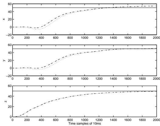
Figure 10: Set-point position control when the initial state is far from the set-point, desired —, strong -.- and weak ... winds.
