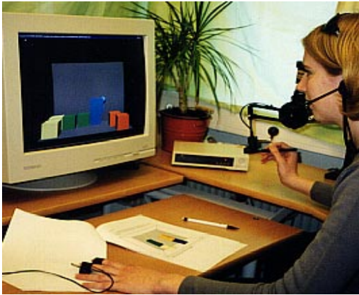
Figure 1. One subject doing task number three with the haptic force feedback device (PHANToM) together with another subject that is in another room.
