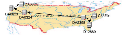
Figure 2. Routing regarding network proximity in PeerCast P2P network
