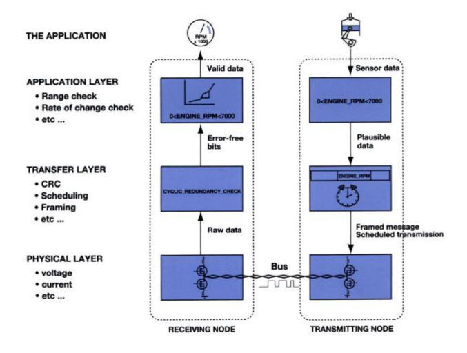
Figure 10. Three layer communications
