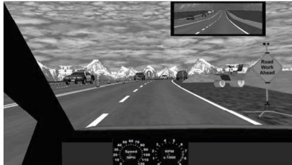
Fig. 3. STISIM Drive – Driving scenario with roadwork and road signs. Note the rear-view mirror located in the top right corner of the picture. Traffic can either be programmed to follow traffic regulations or drive without adherence to traffic regulations
