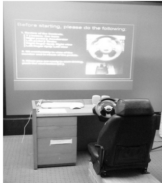
Fig. 1. STISIM Drive - Driving simulator.
