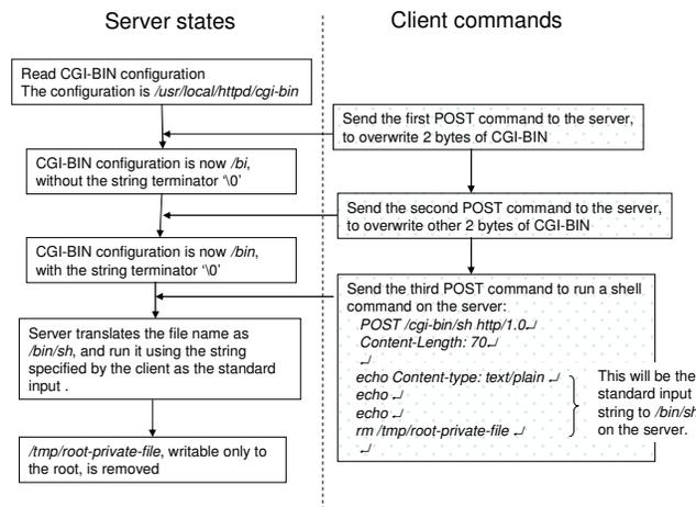
**Figure 2: Configuration Data Attack against NULL HTTPD**
